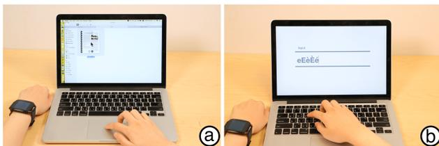
Figure 18. A user can use Dwell+ for fast mode-switching while using a laptop by either inputting through the (a) trackpad or (b) keyboard. The vibration is generated from a smartwatch.
