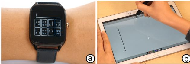
Figure 17. (a) Small-screen text input enabled by Dwell+; each button contains a set of characters which can be selected by a touch. (b) Dwell+ enables fast tool-changing with a stylus on a tablet.
